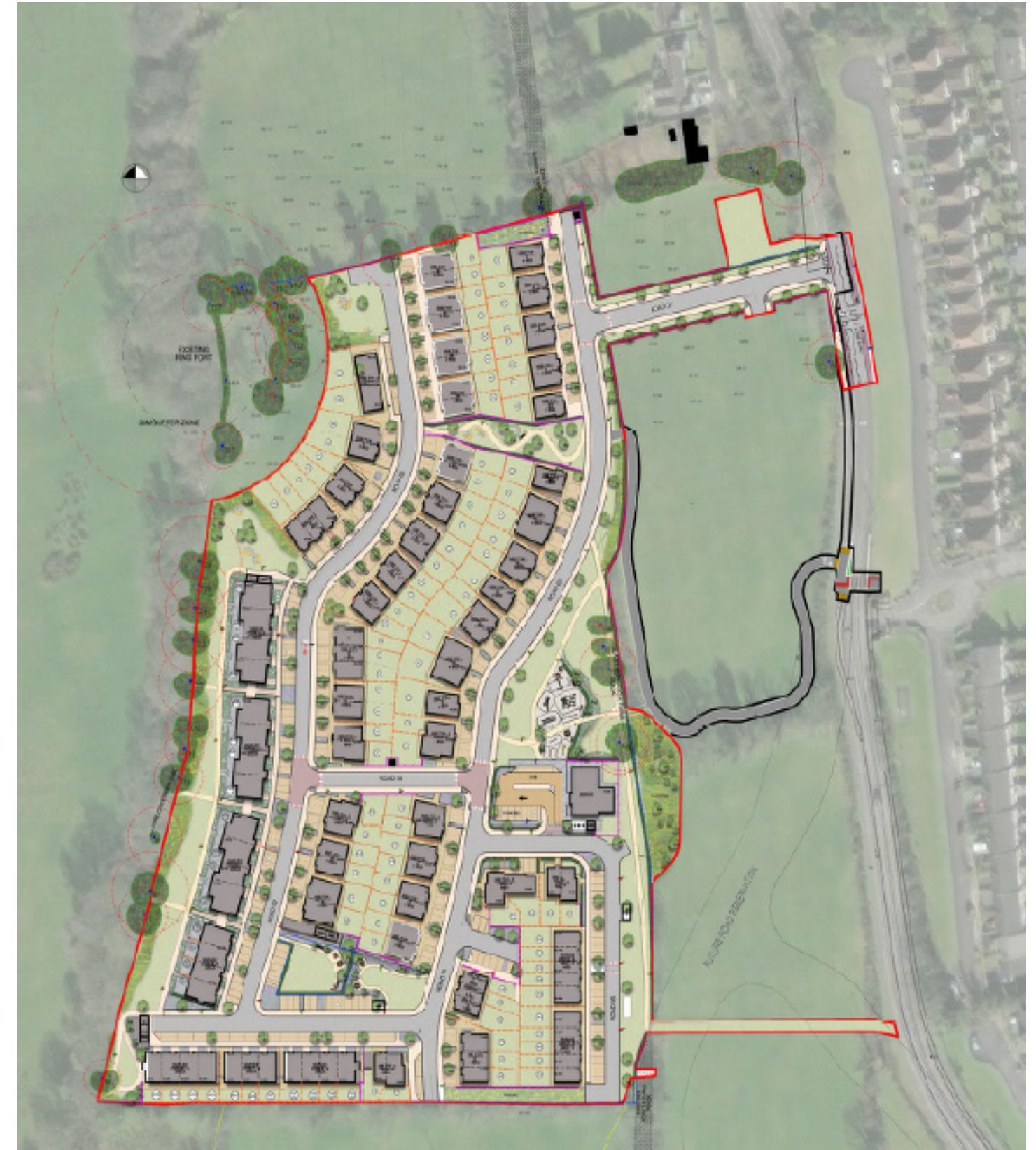
Extract from the site layout which illustrates the block sizes and also how the segregated cycle facilities lead to on-street shared streets for cyclists within the 30km/h residential estate
