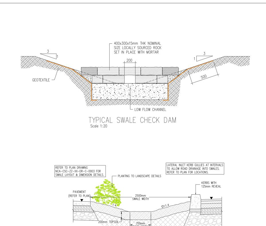
TYPICAL SWALE CROSS SECTION.
